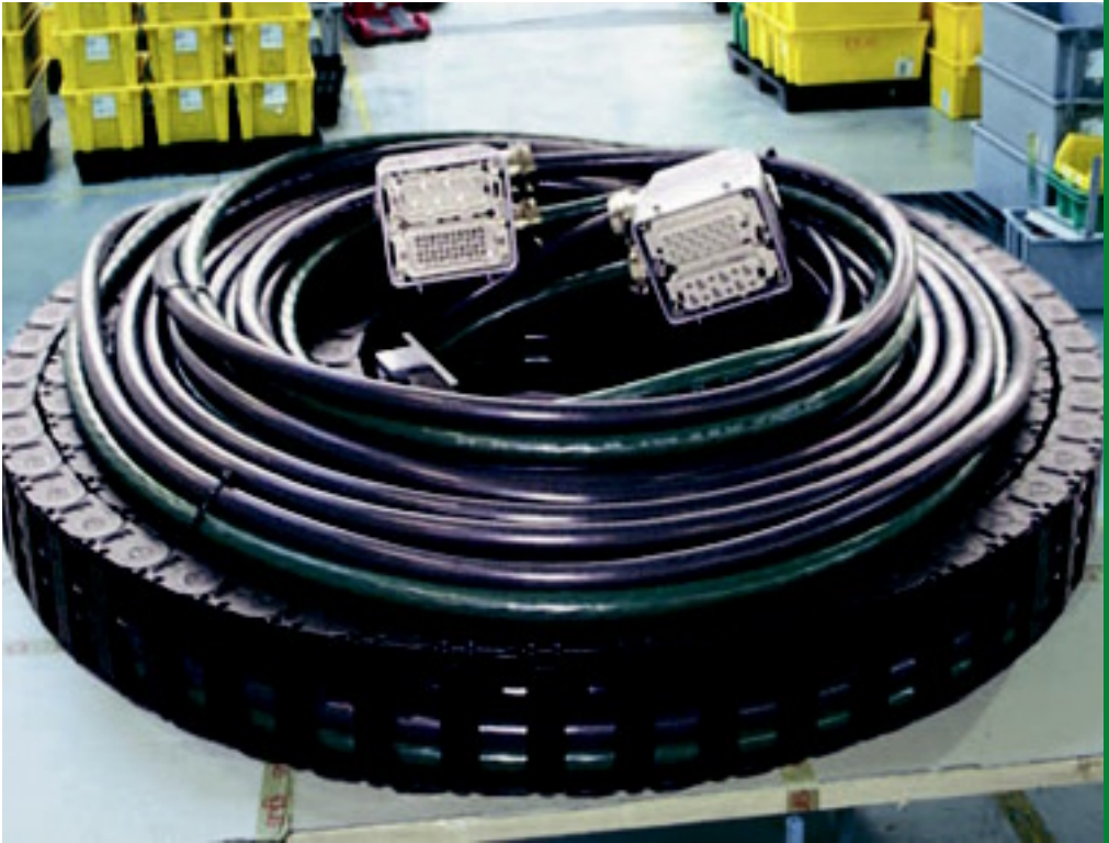
Installation-optimized delivery of an igus® readychain®- here system E2/000
